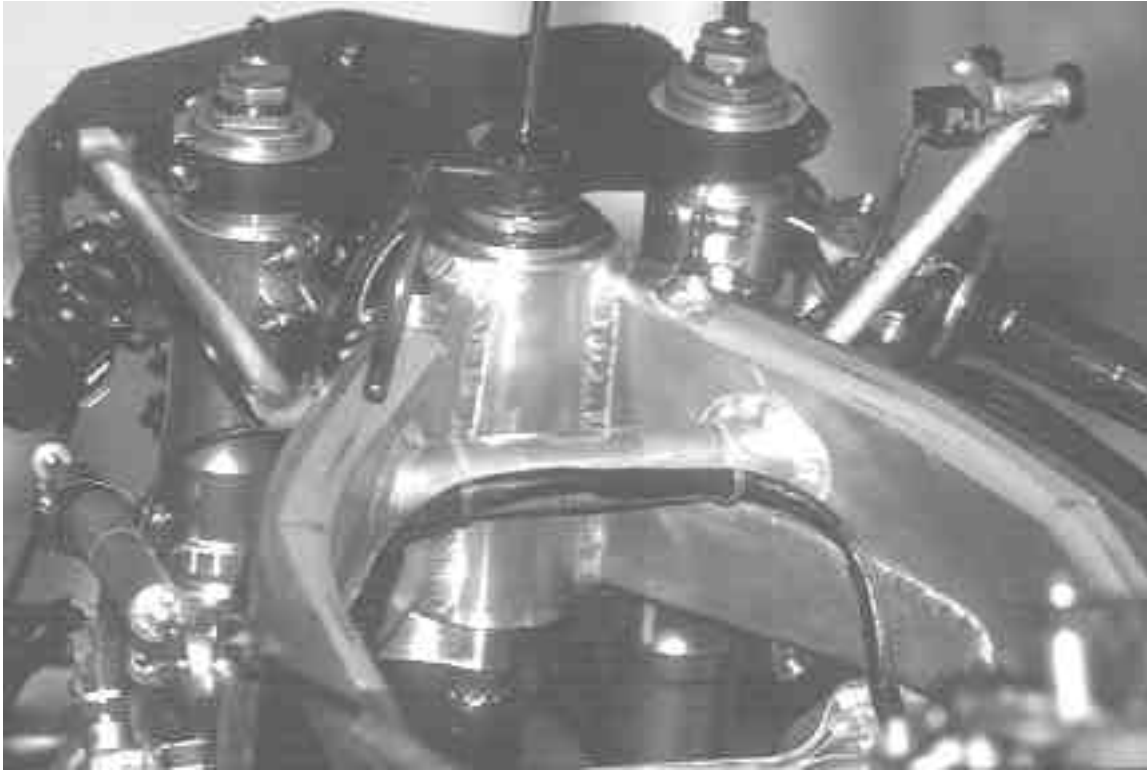
Note how the head stock is supported by the two side beams of this 1997 NSR 250 racing Honda. Frame material is aluminium alloy.
